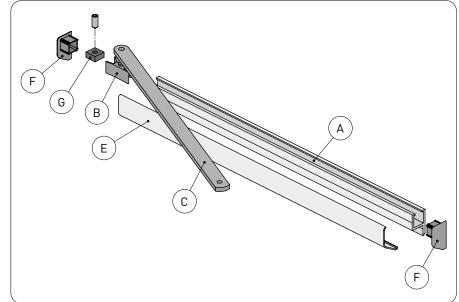
Use the SBS sliding arm for doors which open inward (view from automation side).
