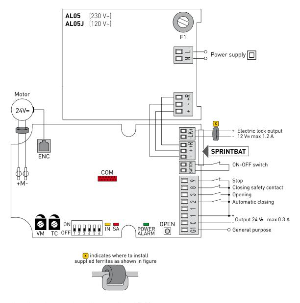
The figure shows the main connections of the control panel EL38.
