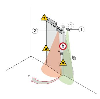
The following safety devices may be installed to protect the danger areas (according to EN 16005):
