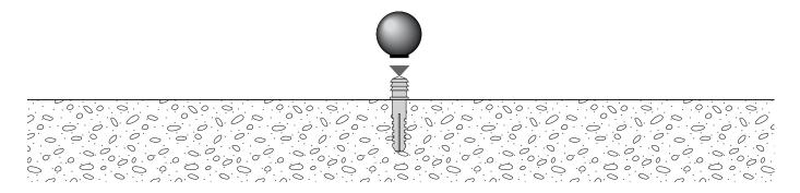
Fasten to the floor the floor doorstop as a mechanical stop in opening.
