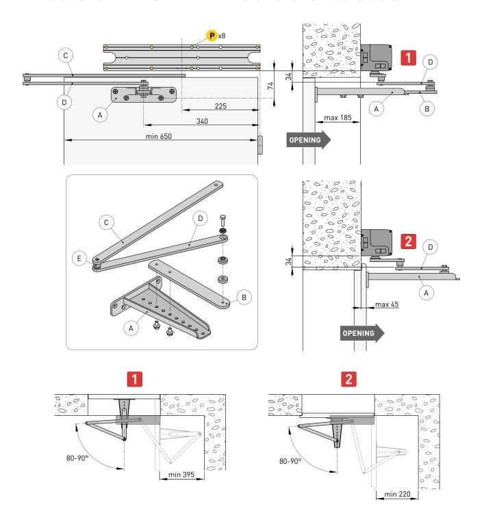
Use the SPRINTBRAS 3-lever articulated arm for doors which open inward (view from automation side).
